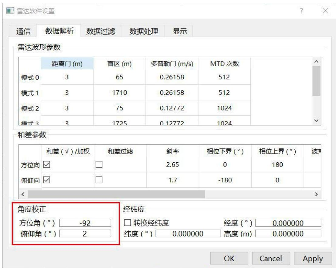
Figure 3.9 Azimuth pitch correction
