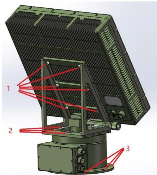
Figure 2.4 Screw mounting position diagram
