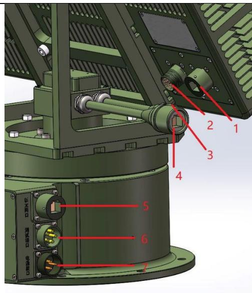
Figure 2.3 Radar interface diagram
